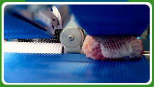
Springout occurs from lengthwise compression during stuffing when the joint is pushed into the netting, causing the meat to spring out of the ends when portioned. Our bespoke roller system pulls the meat, elongating it, enhancing shelf appearance.
