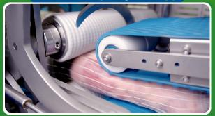
Springback occurs if the netting isn't applied squarely, causing blade cuts to damage multiple rubber strands when portioning. The DS1200AC3's unique centralising roller system ensures an even, square netting application, eliminating springback.
